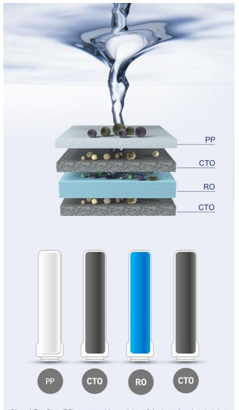
Stage1:Pre-filter (PP) removes big particles of dust, mud and rust stains.
